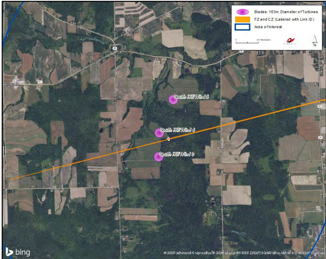
Figure 3: Microwave Paths with Fresnel Zones
